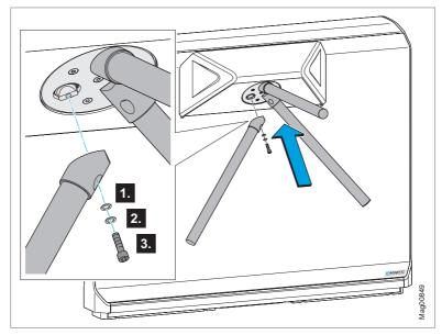
Fig. 33: Mount the blocking arm without the drop arm function. Observe the mounting sequence of the washer, Nordlock washer and hexagon socket screw.
