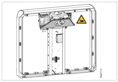
Fig. 28: Mounting the trapezoidal plate
