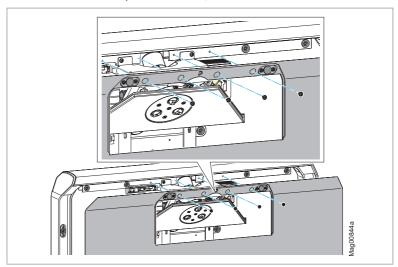
3. Dismount the front panel. To do this, loosen the 4 screws.
