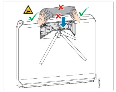
Fig. 35: Mounting the cover
