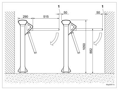
Fig. 3: Clearances and line configuration to be maintained
