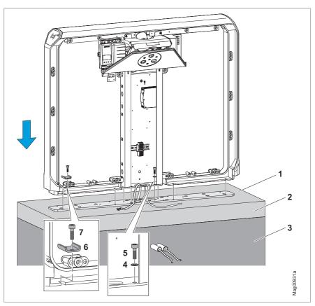
Fig. 26: Mounting variant 3, shown here mTripod FMTP-ML
