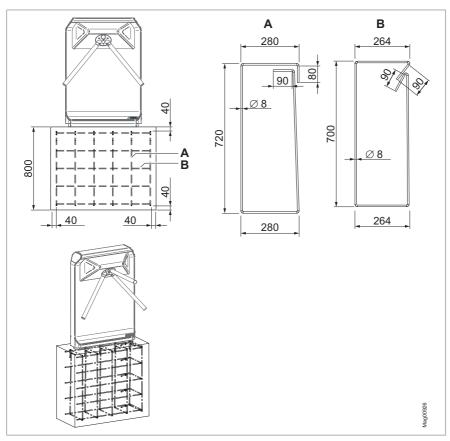
Fig. 9: Reinforcement plan FMTP-MS (dimensions in mm)
