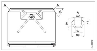
Fig. 39: Installation space for access-control device (dimensions in mm)
