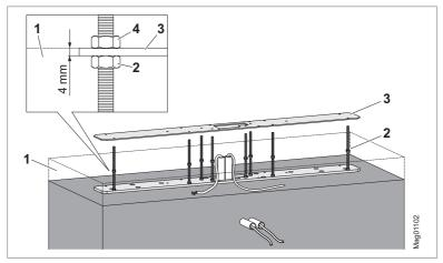
Fig. 19: Positioning the FlowMotion base plate
