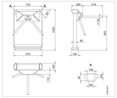
Fig. 2: Dimensions FMTP-MS (dimensions in mm)
