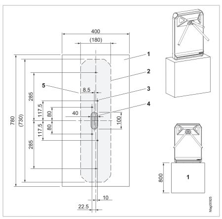
Fig. 8: mTripod FMTP-MS foundation and empty conduit plan (dimensions in mm)
