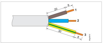
Fig. 37: Stripping (dimensions in mm)
