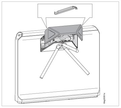
Fig. 34: Dismounting the cover using a tool
