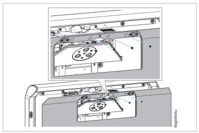
3. Attach the front panel with the 4 screws.
