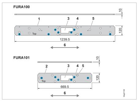
Fig. 10: Base frames FURA100 and FURA101 (dimensions in mm)
