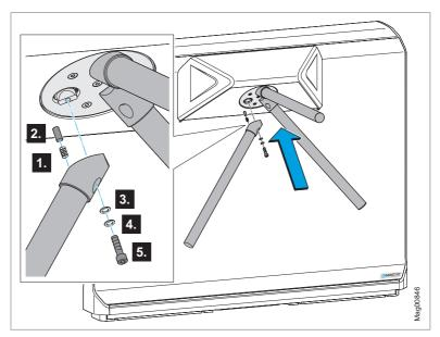
Fig. 32: Mount the blocking arm with drop arm function Observe the mounting sequence of spring, silicone sleeve, washer, Nordlock washer and hexagon socket screw.
