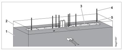
Fig. 18: Mounting the base frame and threaded rods
