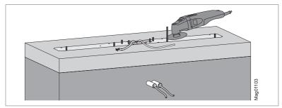
1. Flex off the threaded rods 20 mm above the finished floor.
