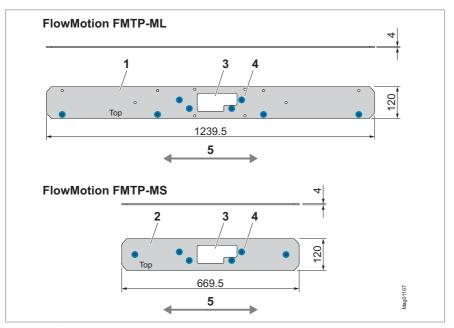
Fig. 11: Base plates FlowMotion (dimensions in mm)
