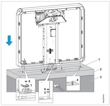
Fig. 22: Mounting variant 2, shown here mTripod FMTP-ML
