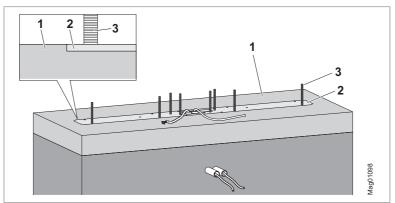
Fig. 20: FlowMotion base plate in the finished floor
