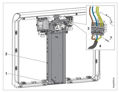
Fig. 38: Laying and connecting the mains cable
