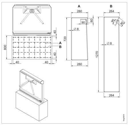
Fig. 7: Reinforcement plan FMTP-ML (dimensions in mm)
