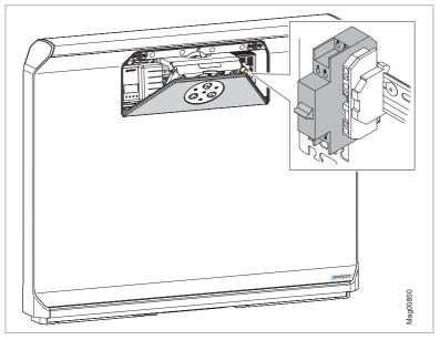
Fig. 41: Switching the mTripod on and off 1 On and off switch
