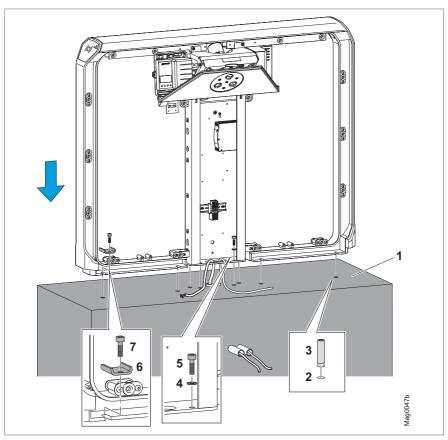
Fig. 17: Mounting variant 1 (direct mounting), shown here mTripod FMTP-ML
