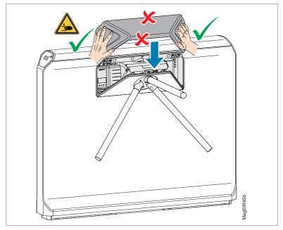
Fig. 31: Mounting the cover
