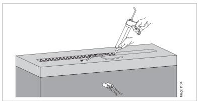
Fig. 24: Applying construction adhesive
