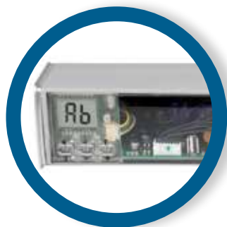
Programming display with 3 keys and USB
