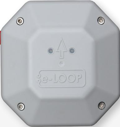
The E-Loop uses magnetometer sensor technology to detect the presence and movement of vehicles. These detections are transmitted to a transceiver for gate activation.
