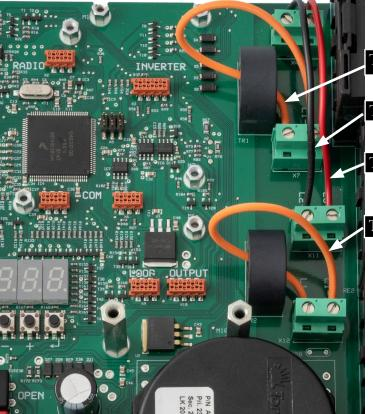
The cable in X7 is removed
