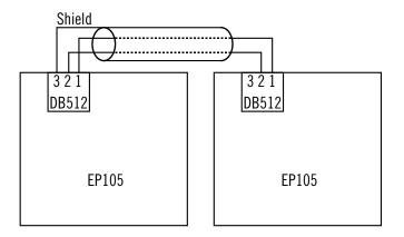
When the card has been installed and connected, the power supply to EP105 can be switched on.
