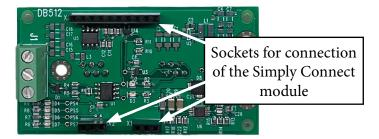
When both the DB512 and the Simply Connect module are mounted, the mains voltage can be switched on to the EP105.
