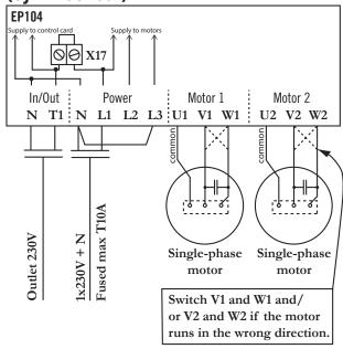
If a symmetrical single-phase motor is used (as shown on the left) make the following changes.
