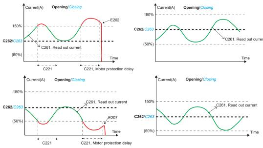
**Load guard:** A swing gate application usually does not require personal protection, if so C240 is set to 0.00. Set C033 to 3, impulse, to activate the load guard. Make sure that the settings of the C242 and C243 is low enough to prevent material damage, but at the same time that it is guaranteed to open due to weather, wind and mechanical changes.
