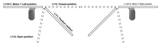
**Motor protection:** Read the motor current during operation in C251 and enter this value in C252 for opening and in C253 for closing. E201 means that the entered value is set too low. E206 means that the entered value is set too high.
