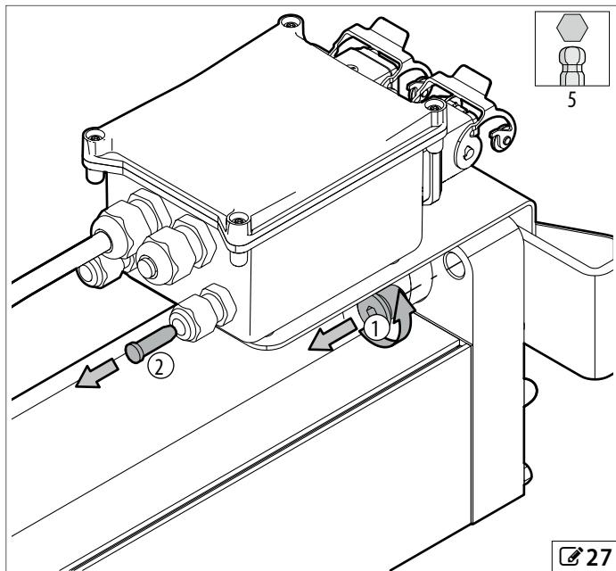
4.  28 Screw the pressure switch 1 onto the flange, together with the seal provided. Insert the cable in to the cable gland 2 and connect it to connector 3 inside the junction box according to the diagram shown in the figure.
