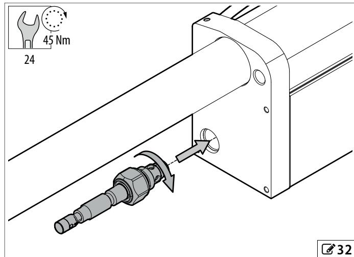
5. Install the control coil onto the solenoid valve.
