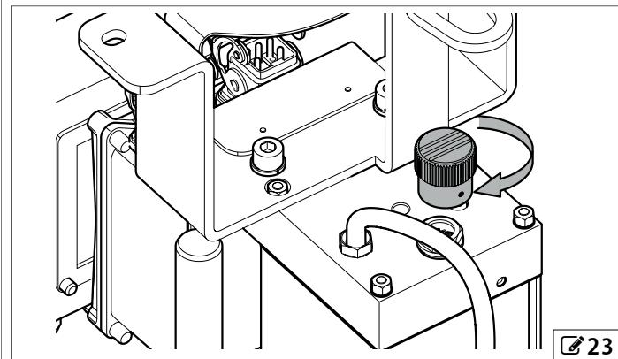
5. Completely remove the hydraulic unit from the bollard.
