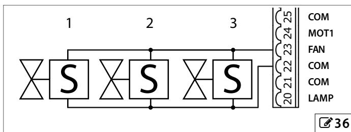
If multiple bollards (more than 3) are installed, which are controlled by JE275 boards in a master / slave configuration, connect the coils to the inputs of the relative control board (master or slave) as indicated in the following diagram.
