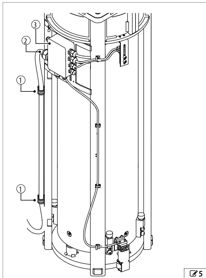
4. Connect the conductors to the external junction box and the control board following the instructions in section § 5.3.
