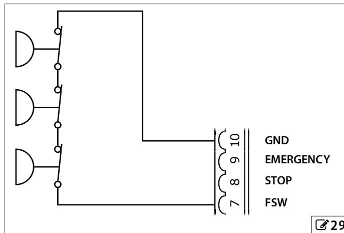
If multiple bollards (more than 3) are installed, which are controlled by JE275 boards in a master / slave configuration, connect all the pressure switches in series on the inputs of the master board as indicated in the following diagram.
