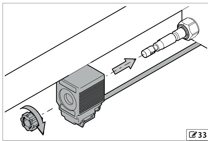
6. Remove the plug from the cable gland **34-1**, insert the cable and connect it to the connector **2** following the indications shown in the diagram.
