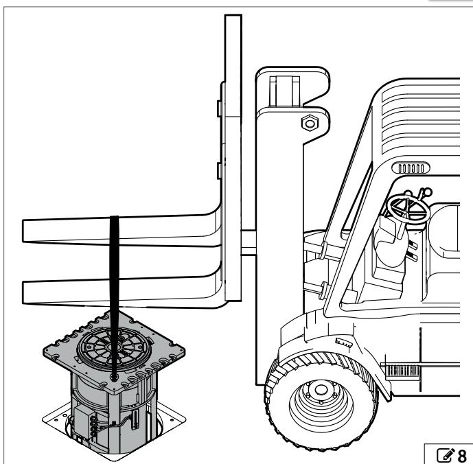
9. Remove the eyebolts and fasten the bollard to the pit using the ten M12x30 screws and the eight M16x30 screws. Apply the fastening torques given in **9**.
