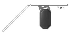
The encoder works by detecting the position of the door, and acts as an intelligent limit switch. A magnetic sensor means that the EP104 knows the precise position of the door, and the limits for the open and closed positions can be directly configured in the unit using degrees, rather than physically changing the limit switch ridges in the motor winder. It is possible to commission one half at a time by activating only one limit switch at a time (L001, L002).
