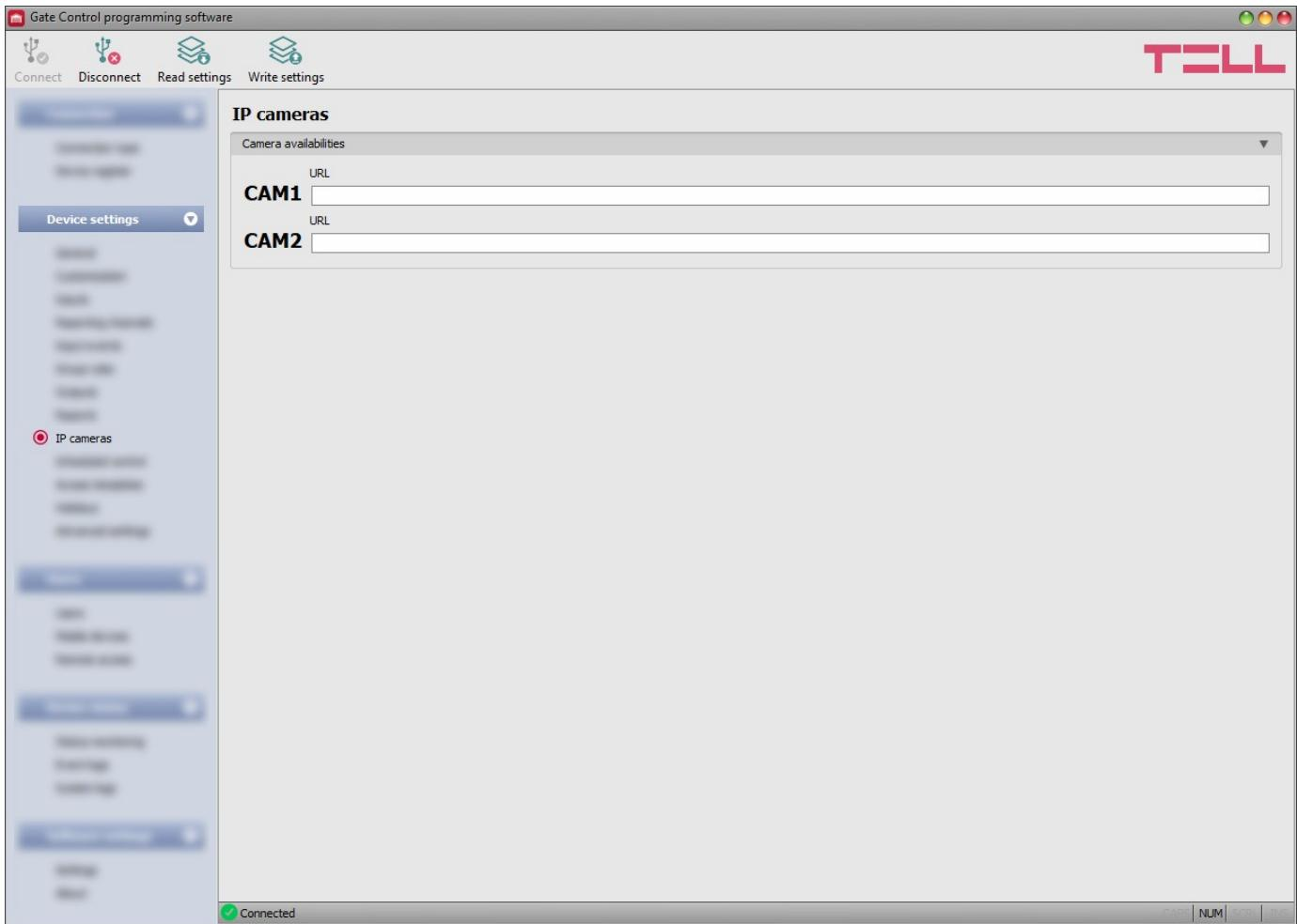
You can configure in the **Gate Control PRO** system the availabilities of up to 2 IP cameras which support the ONVIF standard. The system makes available the pictures of the configured IP cameras in the mobile application. Permission for viewing the camera pictures can be configured for each user and each camera separately in the user settings.
