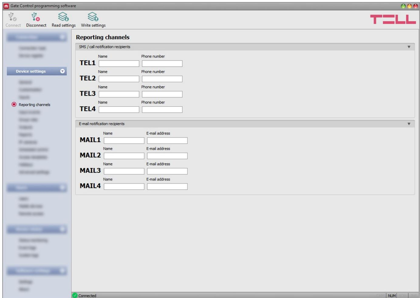
In this menu you can configure the telephone and e-mail availabilities, to which you want to send notifications about events generated by triggering the **IN1...IN4** contact inputs.
