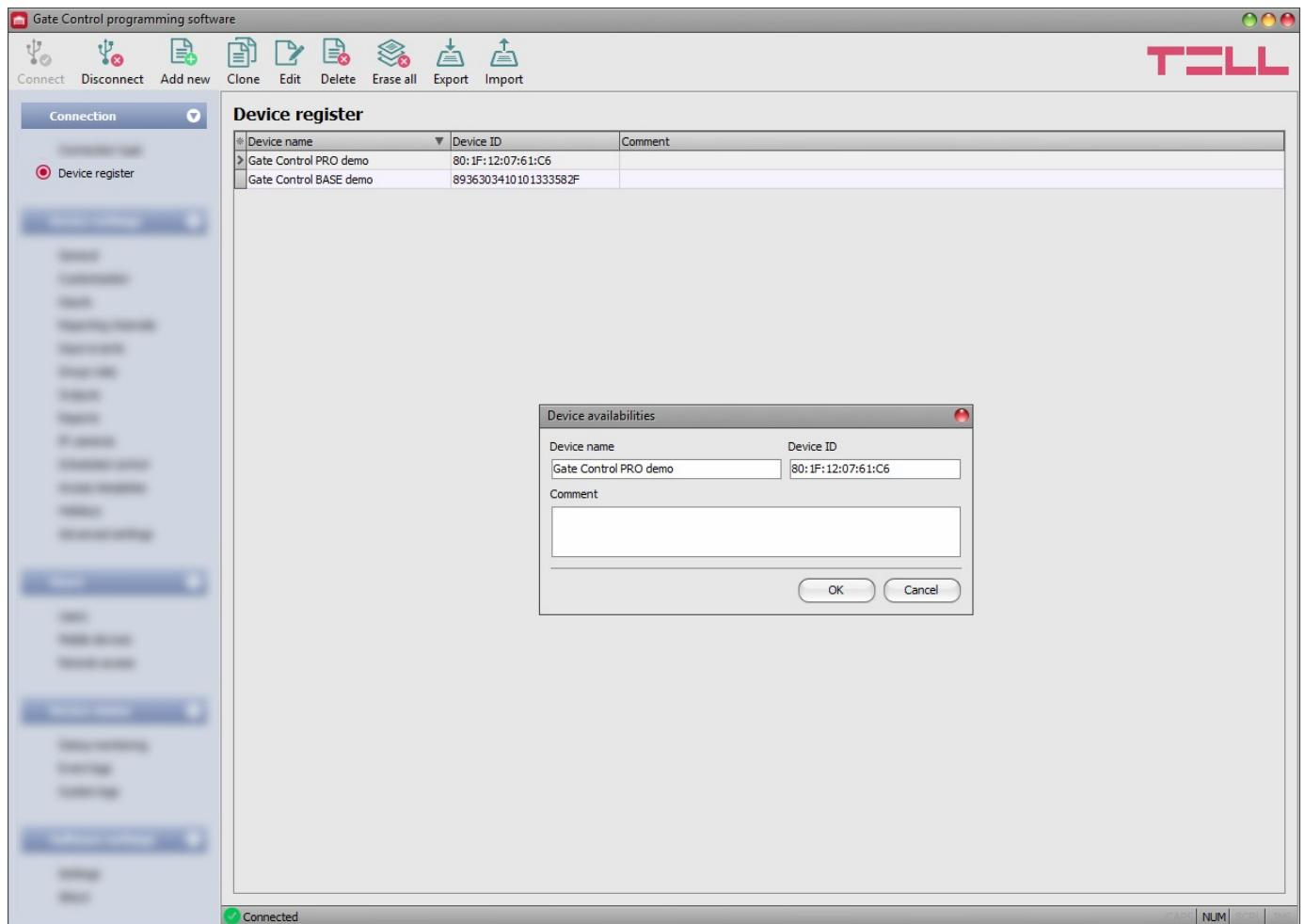
The device register serves for storing and easy management of **Gate Control PRO** and **BASE** device availabilities used for remote access. You can add new device availabilities to the database and also edit, delete and clone entries for easy adding devices with similar availabilities. When connecting remotely, you can easily select by name the device you want to connect to from the "**Device name**" drop-down menu, out of the devices you have added to the database.
