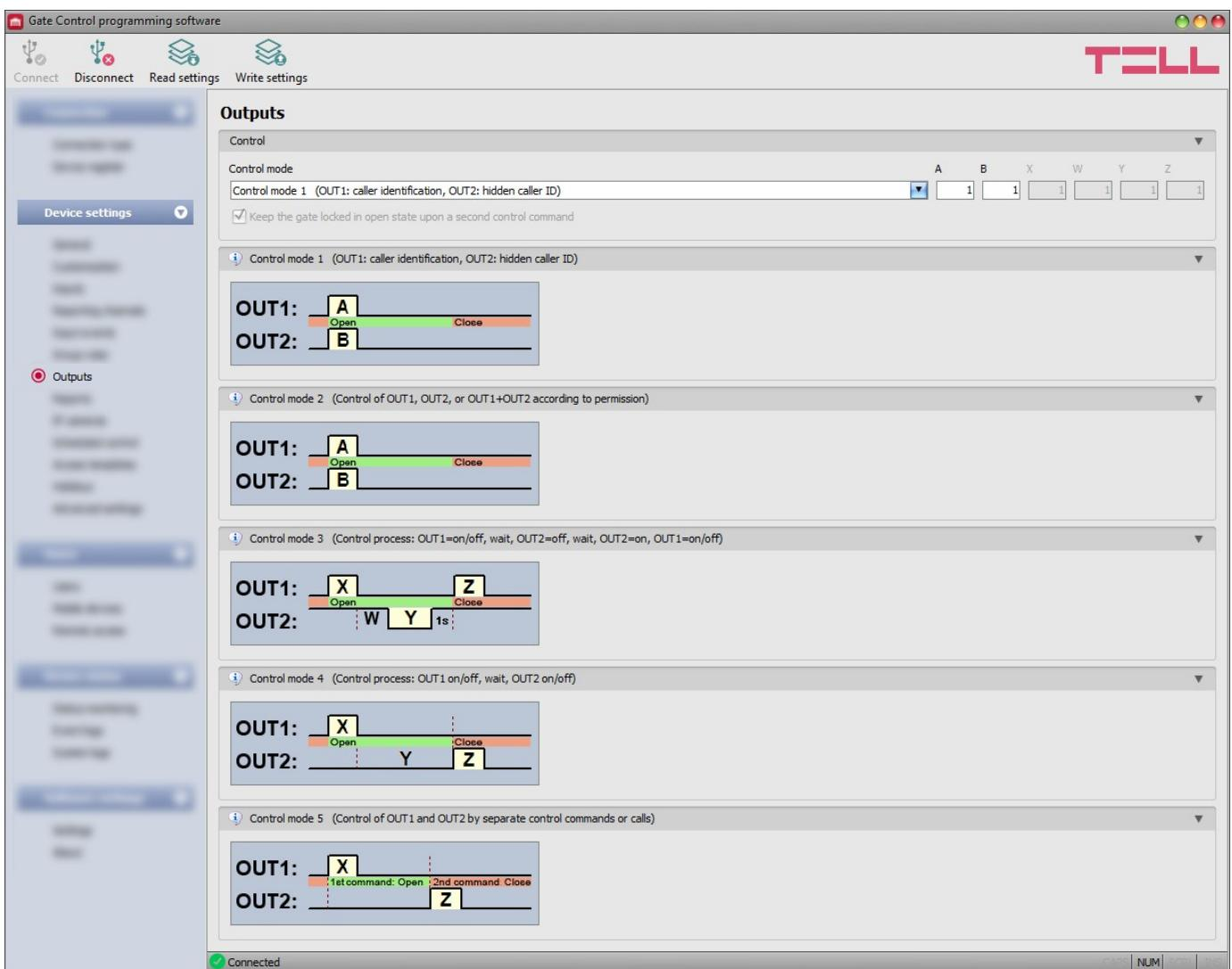
In this menu you can configure how outputs OUT1 and OUT2 should operate when controlled. The operating mode of the outputs can be configured by selecting a control mode. You can choose out of five control modes for compatibility with various control boards of different gates. Choose the control mode which is appropriate for the control signal requirements of the given gate's control board.
