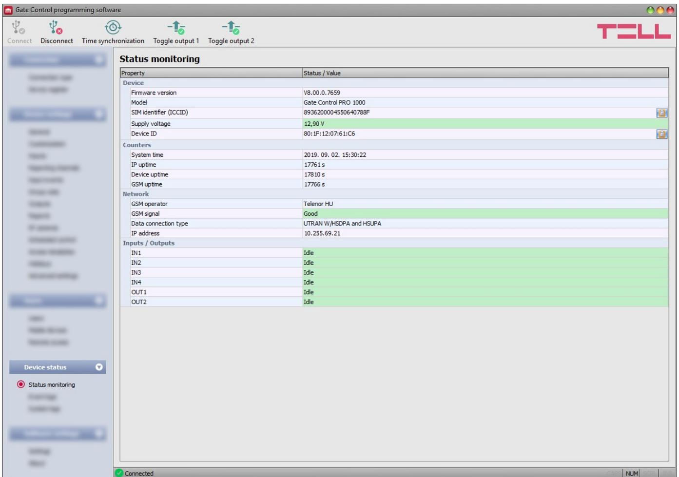
The screenshot shows the 'Gate Control programming software' interface. The top toolbar includes 'Connect', 'Disconnect', 'Time synchronization', 'Toggle output 1', and 'Toggle output 2'. The 'Status monitoring' menu is selected in the left sidebar. The main window displays a table of system properties and their values.
