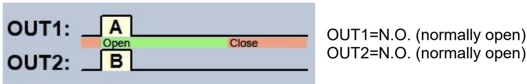
**A** = OUT1 impulse length (seconds) => for opening gate A
