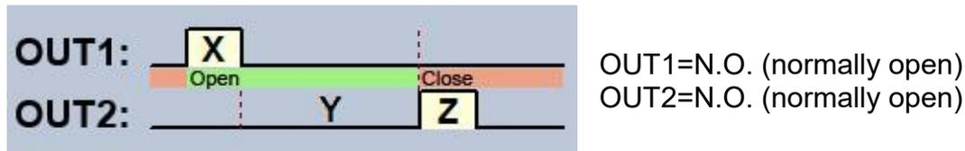
$X$  = OUT1 impulse length (seconds) => for gate opening
