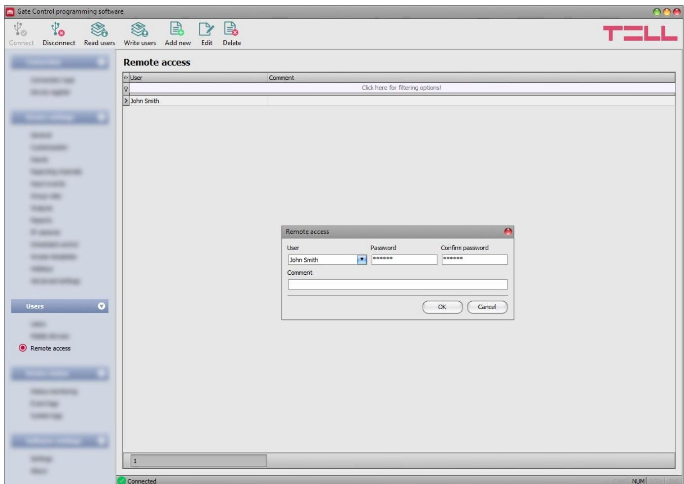
In this menu you can configure passwords for remote access, for super admins and admins. In the possession of the user name and password, the super admin or admin will be authorized to connect to the system remotely over the Internet, using the programming software. You can register altogether up to 2000 mobile devices and remote access passwords in the system, which are distributed dynamically among registered users.
