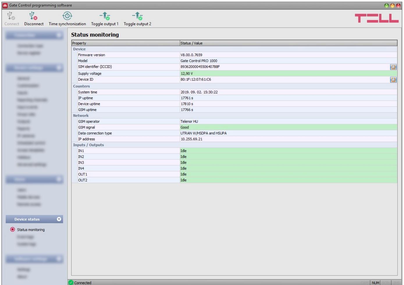
In this menu you can read information about the actual system status. Status information is read from the device and refreshed automatically only when connected through USB. When connected remotely, you can read and refresh the status information by clicking on the “**Read**” button. The availability of certain status information listed below depends on the connected device model.
