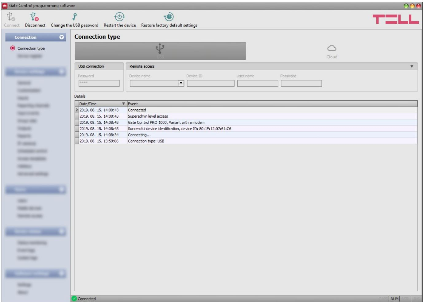
In the “**Connection type**” menu you can select the method of connecting to the device (USB or cloud), view information about the connection process, change the device’s USB password, restart the device, and restore the factory default settings in the device.
