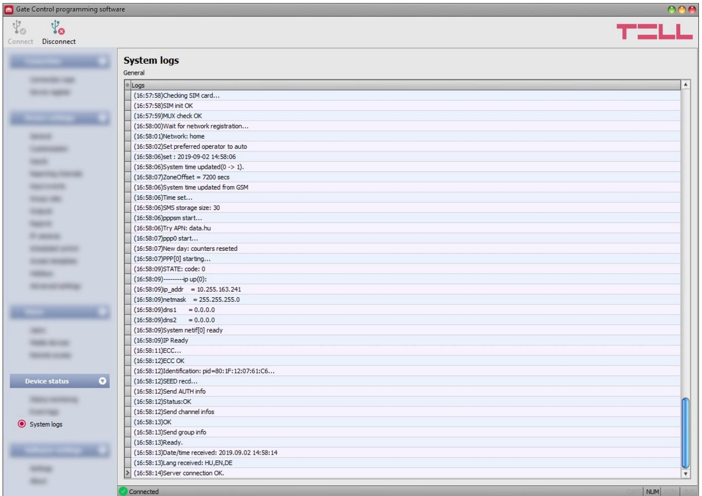
In this section you can view information about the internal processes of the device and communication. These details help troubleshooting if malfunction occurs. **This option is only available when connected through USB!**
