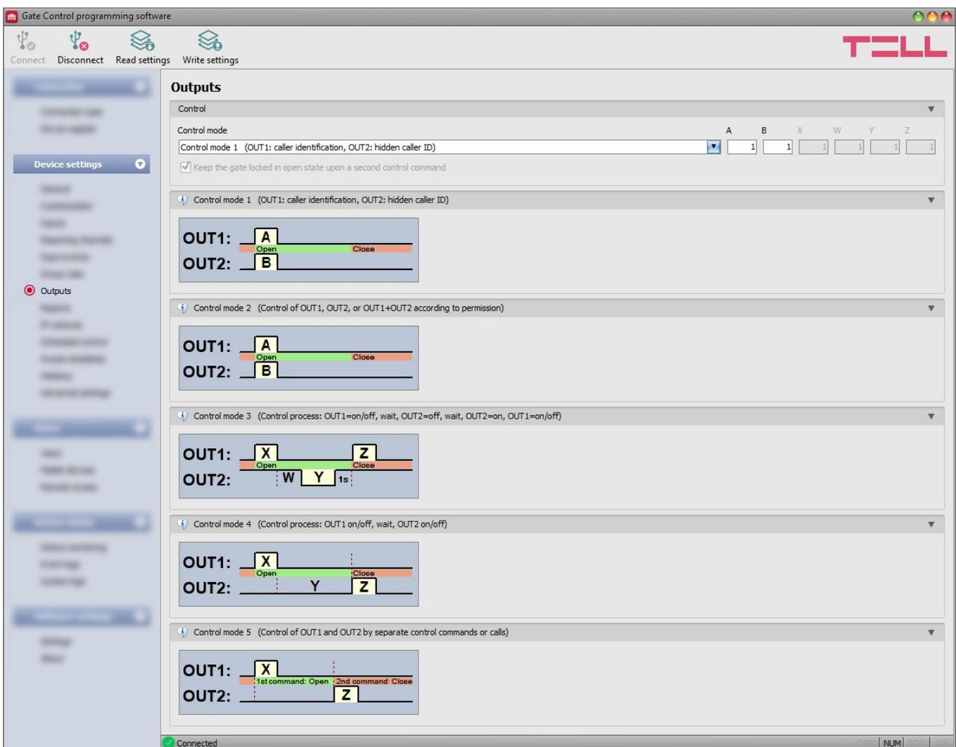
The screenshot shows the 'Gate Control programming software' interface. The 'Outputs' menu is selected in the left sidebar. The main window displays five control modes for configuring outputs OUT1 and OUT2. Each mode includes a timing diagram showing the sequence of events (Open/Close) and the duration of the signal. The control modes are:
