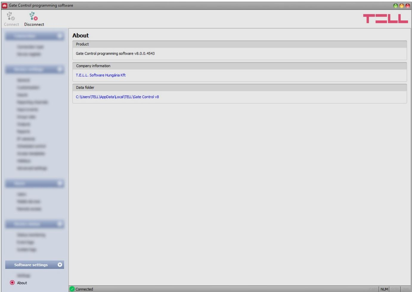
In this menu you can view the availabilities of the manufacturer, the version of the programming software, and the path of the data folder where the software stores system logs. By clicking on the path, the program will open the data folder in the file manager.
