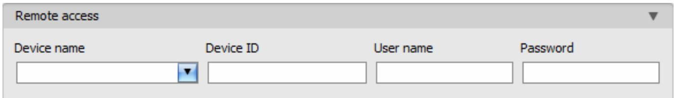
**Device name:** if you have already added the device availabilities in the program's device register, you can select the device you wish to connect to from the drop-down menu.
