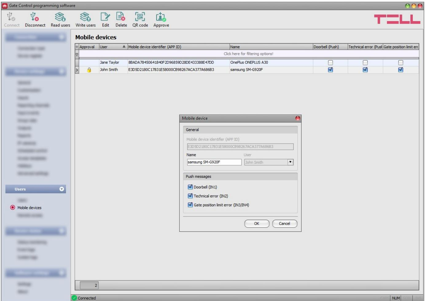
Mobile devices with registered mobile applications and ones waiting for approval are listed in this menu. This is where you can configure which mobile devices shall receive Push notifications. You can register altogether up to 2000 mobile devices and remote access passwords in the system, which are distributed dynamically among registered users. The QR codes used for registering the mobile application are also available in this menu.
