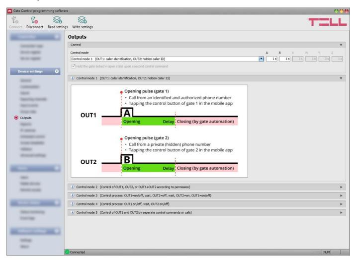
In this menu you can configure how outputs OUT1 and OUT2 should operate when controlled. The operating mode of the outputs can be configured by selecting a control mode. You can choose out of five control modes for compatibility with various control boards of different gates. Choose the control mode which is appropriate for the control signal requirements of the given gate's control board.
