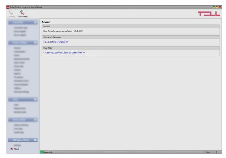
In this menu you can view the contact details of the manufacturer, the version of the programming software, and the path of the data folder where the software stores system logs. By clicking on the path, the program will open the data folder in the file manager.
