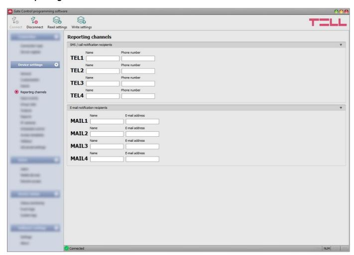
In this menu you can configure the telephone and e-mail contact details, to which you want to send notifications about events generated by triggering the **IN1**...**IN4** contact inputs.
