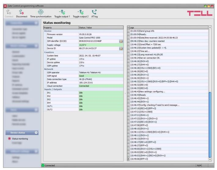
In this menu you can read information about the actual system status. Status information is read from the device and refreshed automatically only when connected through USB. When connected remotely, you can read and refresh the status information by clicking on the "*Read*" button. The availability of certain status information listed below depends on the connected device model.
