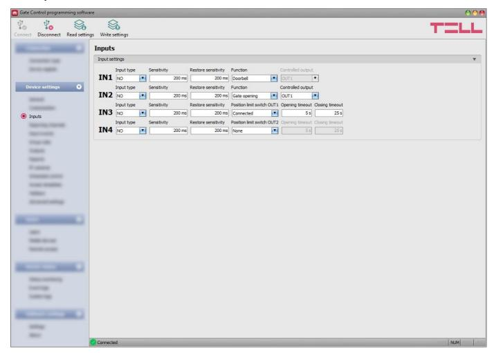
In this menu you can configure the properties and options of the contact inputs IN1...IN4. When the contact inputs are triggered, the system generates input events. You can configure notifications for each input event in the "*Input events*" menu, which will be sent to the phone numbers and/or e-mail addresses configured in the "*Reporting channels*" menu. In addition, the inputs have further configurable functions, as follows:
