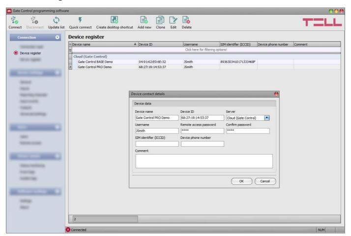
The device register serves for storing and easy management of *Gate Control PRO* and *BASE* device contact details used for remote access. You can add new device contact details to the database and edit, delete, and clone entries for easy adding devices with similar contact details. When connecting remotely, you can easily select by name the device you want to connect to from the "*Device name*" drop-down menu, out of the devices you have added to the database.
