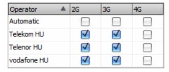
**Network selection**: the mobile network management in the device is automatic by default. If you experience problems with the stability of the mobile network in the given location, that is the device switches frequently between networks, you can select manually the network you want to use.
