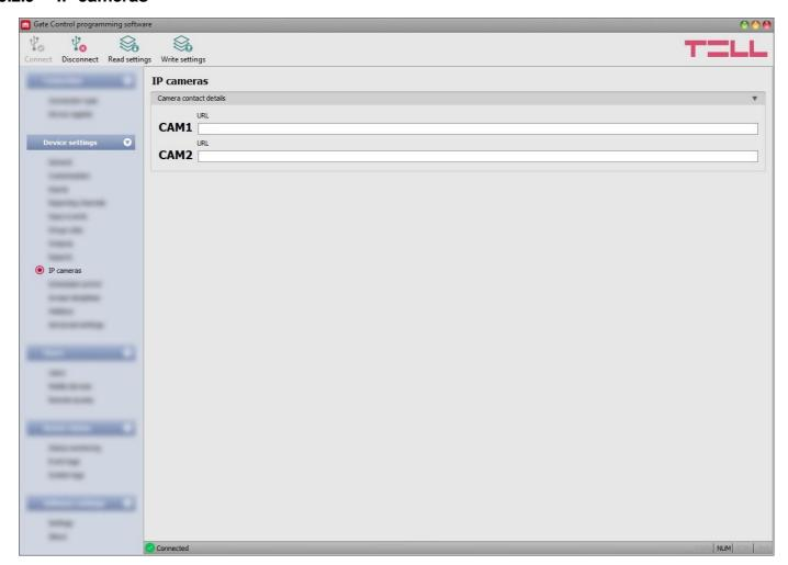
You can configure in the *Gate Control PRO* system the contact details of up to 2 IP cameras which support the ONVIF standard. The system makes available the pictures of the configured IP cameras in the mobile application. Permission for viewing the camera pictures can be configured for each user and each camera separately in the user settings.
