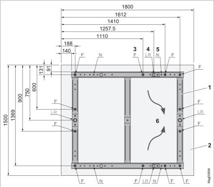
Fig. 10: Foundation and empty conduit plan for base frame FURA T3 – top view (dimensions in mm)
