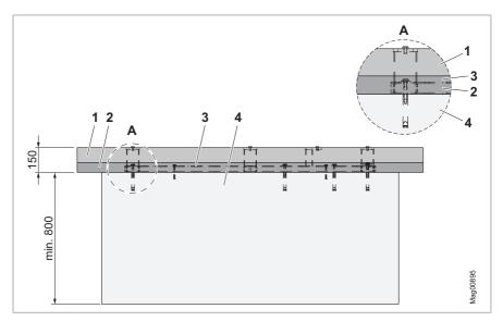
Fig. 11: Foundation and empty conduit plan for base frame FURA T3 – side view (dimensions in mm)
