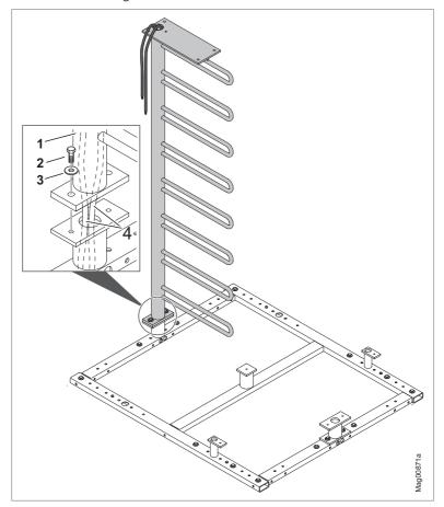
Fig. 16: Installing the locking comb
