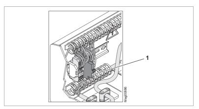
Fig. 34: Switching MPT-333 on and off
