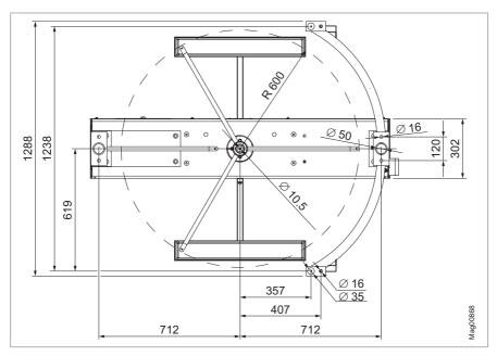
Fig. 3: Dimensions MPT-333 - view from below (dimensions in mm), lighting optional
