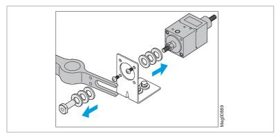
Fig. 39: Remove magnet, washers and union nut
