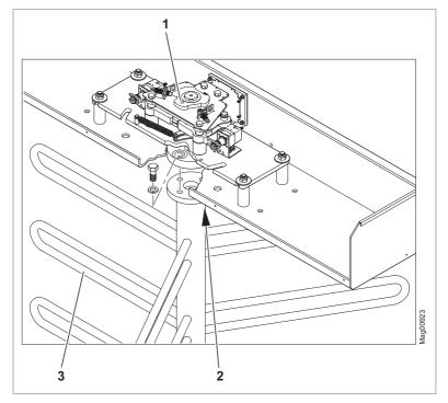
Fig. 21: Correct positioning of the locking unit – illustration shows version "Entrance side right"; in version "Entrance side left", the centre pillar is turned by 180°.
