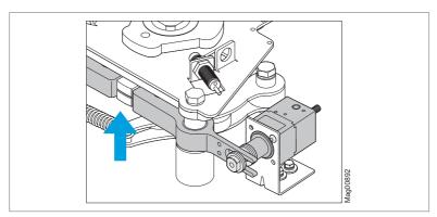
Fig. 42: Locking unit configuration "Normally closed"
