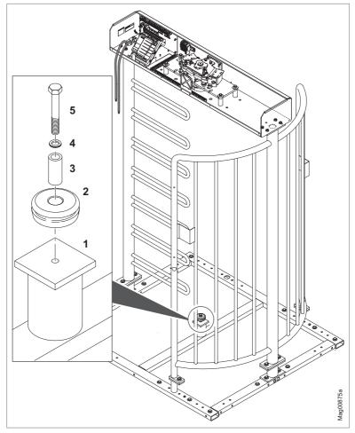
Fig. 19: Mount floor bearing (plastic bearing, sleeve, washer and hexagon head screw)
