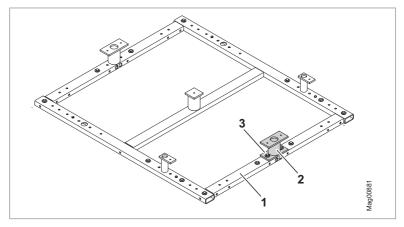
Fig. 14: Assemble base frame FURA T3
