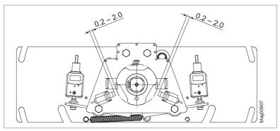
Fig. 36: Distance proximity sensor - switching cam
