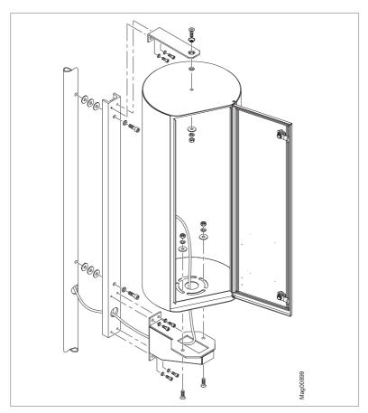
Fig. 24: Mounting pillar and attachment material
