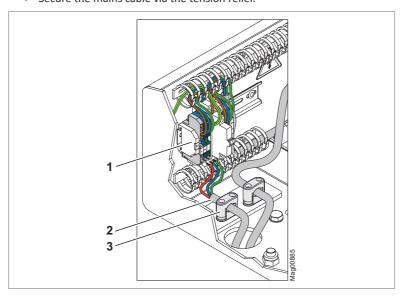
Fig. 33: Connecting the mains cable
