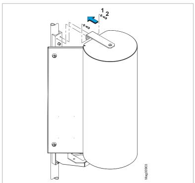
Fig. 28: Mounting the attachment angle
