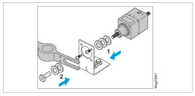
Fig. 41: Mount magnet, washers and union nut (normally open)
