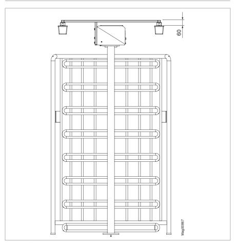
Fig. 2: Dimensions MPT-333 - side view (dimensions in mm), lighting optional
