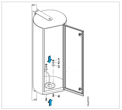
Fig. 30: Fixing the mounting pillar
