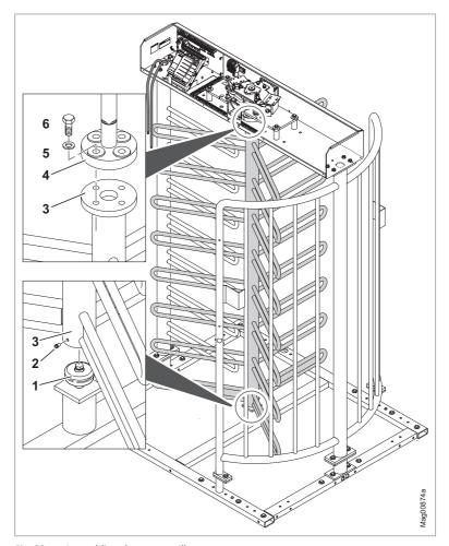
Fig. 20: Assembling the centre pillar
