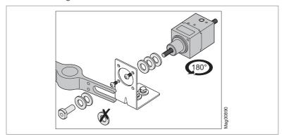
Fig. 40: Turn magnet, remove washer
