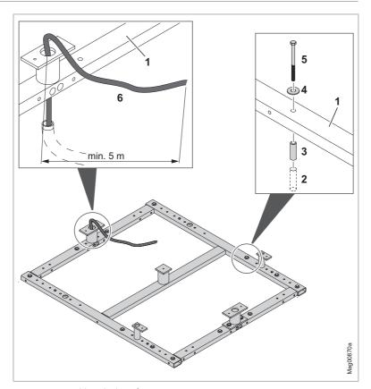
Fig. 15: Assembling the base frame FURA T3
