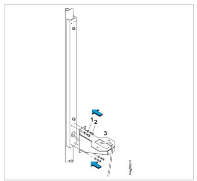
Fig. 26: Mounting the lower holder
