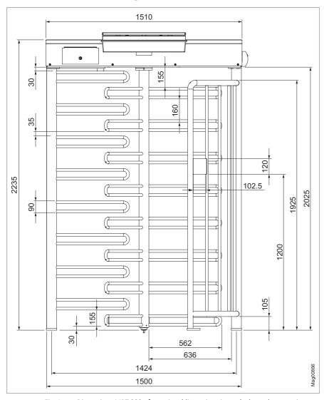
Fig. 1: Dimensions MPT-333 - front view (dimensions in mm), shown here version "entrance side left", lighting optional
