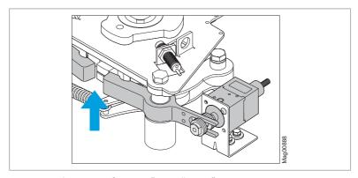
Fig. 38: Locking unit configuration "Normally open"
