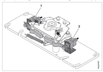
Fig. 37: Locking unit configuration "Normally open"
