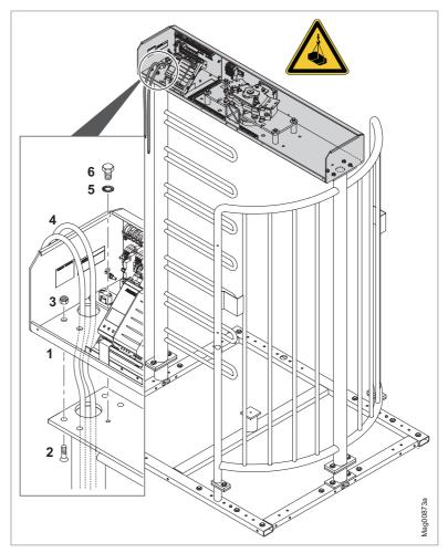
Fig. 18: Putting on the support beam and installing it.
