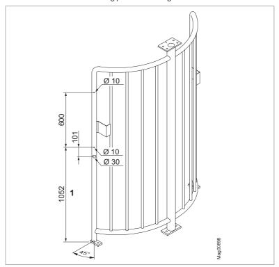
Fig. 23: Required holes mounting pillar (all dimensions in mm)
