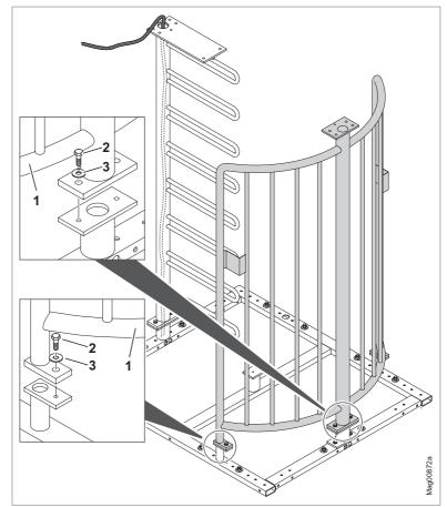
Fig. 17: Installing the cage half
