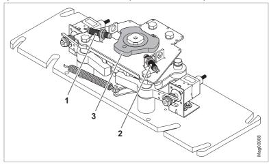
Proximity sensors for detecting the end position of the centre pillar
