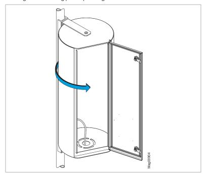
Fig. 29: Aligning the mounting pillar
