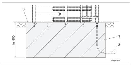
Fig. 13: Foundation and empty conduit plan for direct mounting – side view (dimensions in mm)
