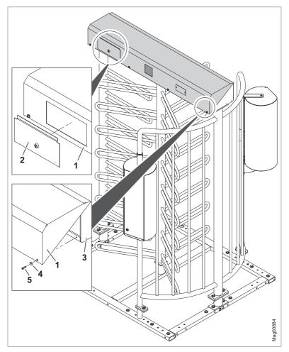
Fig. 31: Open and close cover or service door
