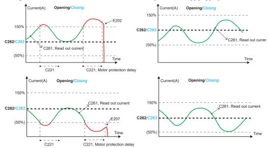
**Load guard:** A swing gate application usually does not require personal protection, if so C240 is set to 0.00. Set C033 to 3, impulse, to activate the load guard. Make sure that the settings of the C242 and C243 is low enough to prevent material damage, but at the same time that it is guaranteed to open due to weather, wind and mechanical changes.
