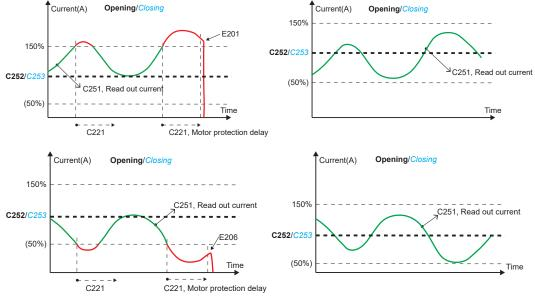
**Load guard:** A swing gate application usually does not require personal protection, if so C230 is set to 0.00. Set C033 to 3, impulse, to activate the load guard. Make sure that the settings of the C232 and C233 is low enough to prevent material damage, but at the same time that it is guaranteed to open due to weather, wind and mechanical changes.
